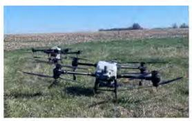
Figure 1. T40 drones equipped with sprayers.
