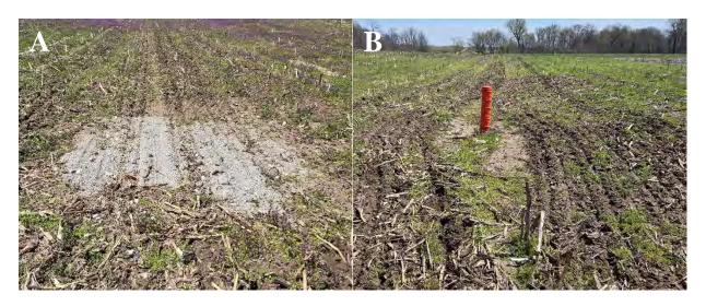
Figure 3. Unobstructed path observed in A) Blind Inlet, but obstruction in B) HickenBottom.
