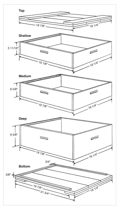
Figure 4. Some parts of a Langstroth hive.
