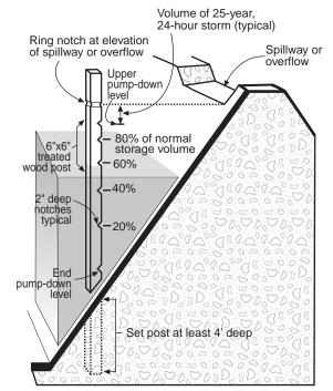
Figure 4. Pump-down marker in an anaerobic lagoon.
