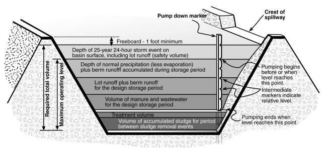
Figure 1. Schematic of volume fractions in lagoon design.
