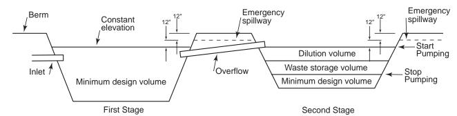
Figure 5. A two-stage anaerobic lagoon designed for the treatment of livestock manure.
