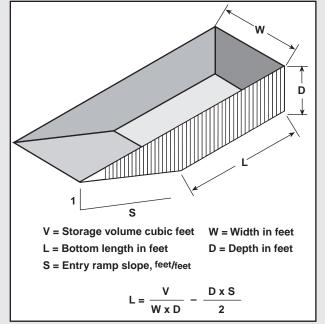
Figure 12. Dimension equation for a picket dam storage facility.
