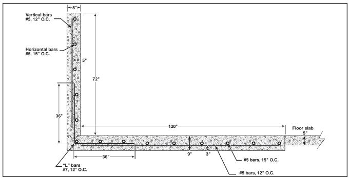
Figure 5. Design for a six-foot free-standing concrete wall.
