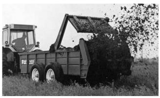
Figure 2. This box-type spreader is equipped with a chain-driven conveyor to move solid manure to the beaters for rear discharge.
