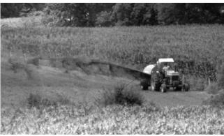
Figure 4. This tank-type applicator is broadcasting slurry onto the soil surface.
