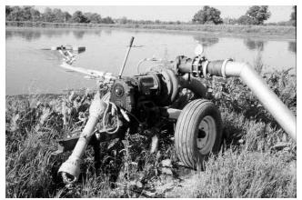
Figure 8. This PTO-powered, high-pressure centrifugal pump fed by a submersible chopper pump, is typical of pumps used with irrigation systems and drag-hose applicators handling slurry manure.
