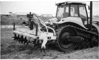
Figure 7. The aggressiveness of this incorporating applicator can be increased by angling the tine shaft.
