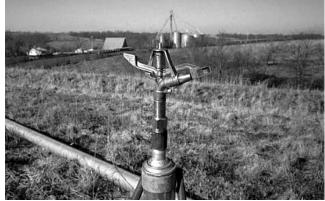
Figure 14. Small sprinklers (up to  $\frac{3}{4}$ -inch diameter) can be used to irrigate lagoon effluent onto irregularly shaped fields.
