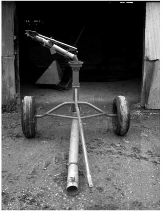
Figure 16. Stationary big gun on wheels to facilitate moving.
