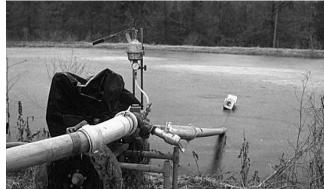
Figure 9. To prevent intake of floating debris, suspend an irrigation pump intake about 2 feet below the surface of a lagoon.
