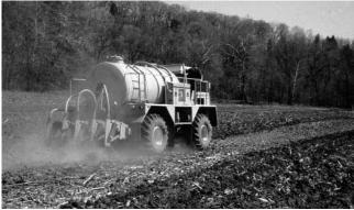
Figure 5A. This self-propelled, tank-type applicator is equipped to inject slurry below the soil surface, thus reducing nutrient losses and odor emissions.
