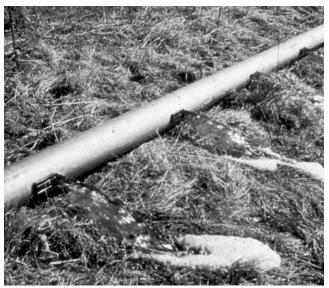
Figure 20. Gated pipe systems are occasionally fed by gravity from a lagoon at a higher elevation.
