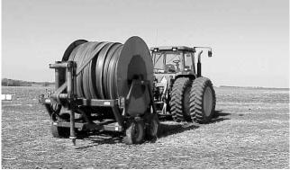
Figure 12. Hose carts provide a compact, fast means to transport, lay out and take up flexible drag hose or feeder hose.
