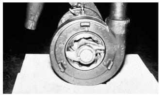
Figure 10. Chopper blades on the intake of a centrifugal pump.
