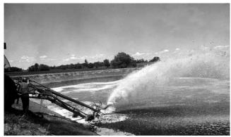
Figure 11. This PTO-powered, high-capacity pump can either fill tankers or bypass effluent to agitate a lagoon, or both.
