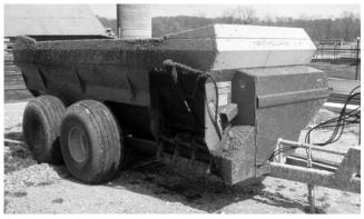
Figure 3. This side-discharge, hopper-type spreader can be used for solid and semisolid manure.
