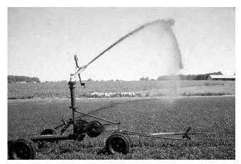
Figure 17. Soft-hose traveling big gun irrigators are frequently the system of choice for land application of lagoon effluent.
