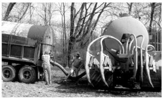
Figure 5B. The self-propelled, tank-type applicator shown in Figure 5A is being refilled from a tender truck.
