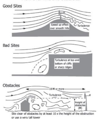
Credit: DOE NREL Figure 1. An illustration of how turbulence affects different sites.
