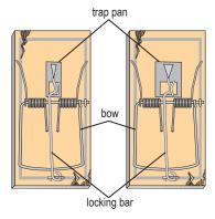
Figure 3. Snap traps with larger trap pans are also available and allow for more bait to be used. They are easier to set than normal traps, and some have a sensitivity setting that prevents the trap from snapping prematurely.
