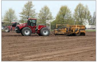
**Figure 22.** GPS guided land grading is used to improve drainage and uniformity of water application with furrow irrigation.
