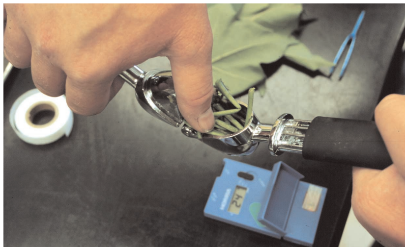
Figure 44. Using a Cardy® meter to test nitrate in cotton plants begins with extracting sap from cotton petioles with a garlic press.
