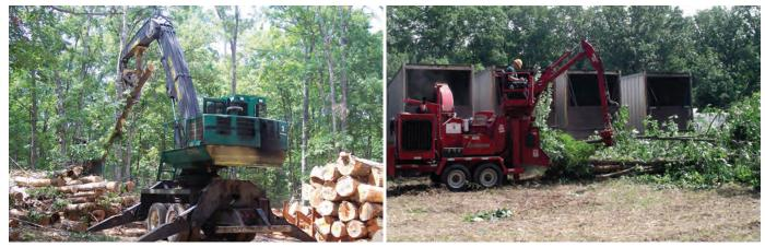
Figure 7. An integrated, one-pass harvest sorts and processes low-value woody biomass at the landing.
