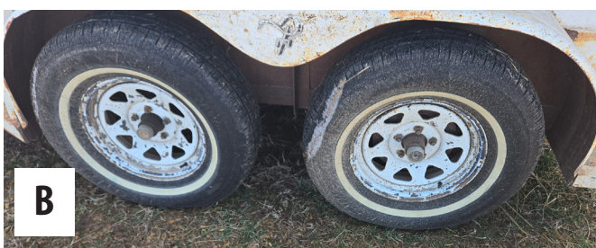
Figure 5. Always check the integrity of your trailer tires before hauling. Look for cracking, dry rotting, bald tires, or low tire pressure. Figure 5A displays a tire with significant dry rot, which increases the risk of a blowout. Like Figure 5B, many tires will lose air pressure when temperatures drop in the winter and may need to be filled to pull efficiently.
