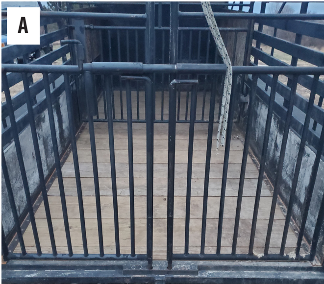
Figure 4. In Figure 4A, this trailer does not have floor mats, making it easier for the owner to identify rot or potential safety issues if they arise. In Figure 4B, this trailer does have mats, therefore, periodically, you should lift mats in your trailer to check on the integrity of your floorboards. Look for dark areas that indicate water damage and soft or rotten boards. This is also a great time to evaluate the metal framing holding the floorboards for any rusting or damage that could pose a safety risk. While mats can be useful for traction or stability, you need to check floorboards regularly because trapped moisture from rain or urine can cause rot or damage to your floorboards without being noticed.
