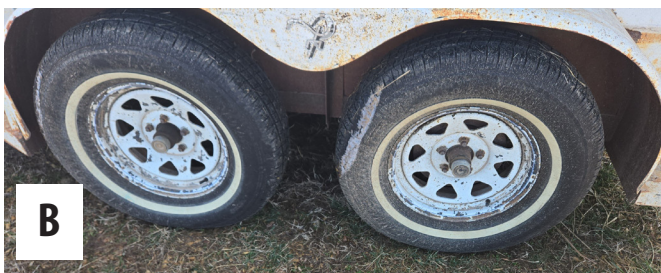
Figure 5. Always check the integrity of your trailer tires before hauling. Look for cracking, dry rotting, bald tires, or low tire pressure. Figure 5A displays a tire with significant dry rot, which increases the risk of a blowout. Like Figure 5B, many tires will lose air pressure when temperatures drop in the winter and may need to be filled to pull efficiently.
