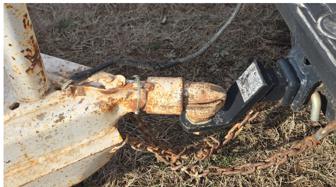
Figure 3. Make sure that you use a properly sized ball to fit the trailer hitch. An under-sized ball is more likely to have the hitch pop off the ball during hauling. A safety pin should also be used to prevent the hitch from coming open and disconnecting from the ball. Safety chains should also be checked for broken welds or damage. For bumper pull trailers, make sure that your safety chains will not drag the ground.
