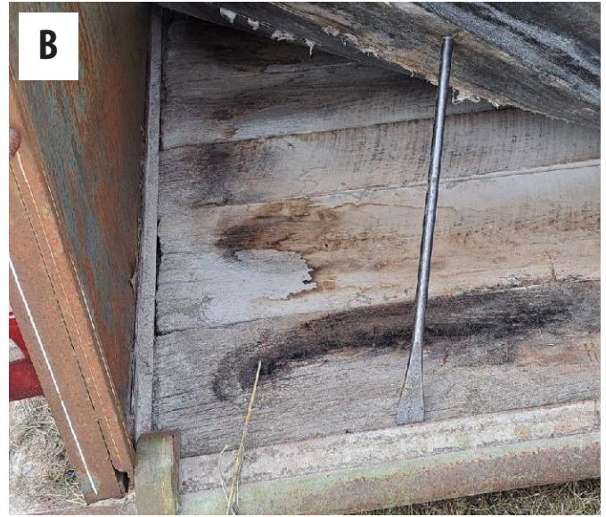
Figure 4. In Figure 4A, this trailer does not have floor mats, making it easier for the owner to identify rot or potential safety issues if they arise. In Figure 4B, this trailer does have mats, therefore, periodically, you should lift mats in your trailer to check on the integrity of your floorboards. Look for dark areas that indicate water damage and soft or rotten boards. This is also a great time to evaluate the metal framing holding the floorboards for any rusting or damage that could pose a safety risk. While mats can be useful for traction or stability, you need to check floorboards regularly because trapped moisture from rain or urine can cause rot or damage to your floorboards without being noticed.
