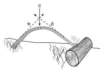
Figure 4. To locate the apex of the bend, imagine straight lines (a and b) coming out of the bent springpole. These lines intersect at some point away from the tree. Draw a third line (c) that bisects the angle formed by lines a and b. Cut where line c touches the top of the springpole.
