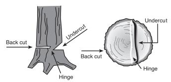
Figure 3. The direction a tree falls can be closely controlled with properly made undercuts and back cuts.
