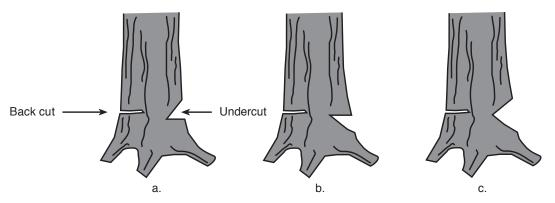
Figure 2. Three types of undercuts. Note that in each case, the back cut is slightly (1 to 2 inches) above the hinge point of the undercut.
