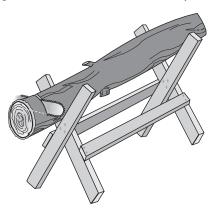
Figure 6. A sawbuck is useful for safely cutting wood to length.
