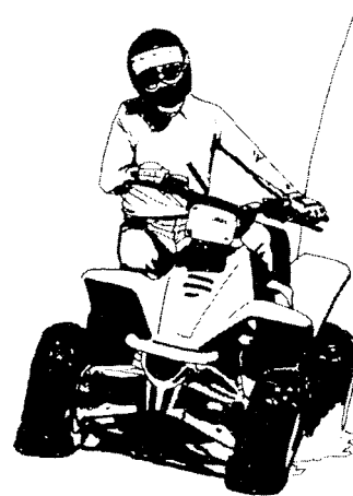
Figure 4. Keep both feet firmly on the footrests and lean your body uphill when crossing slopes.
