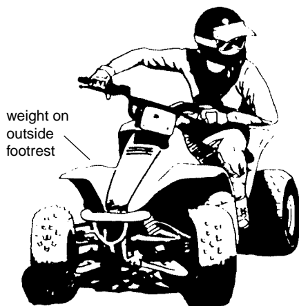
Figure 1. When turning, lean your upper body toward the inside of the turn while keeping your weight on the outer footrest.
