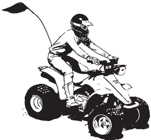
Figure 3. Shift into low gear and point the ATV directly downhill when descending a slope.
