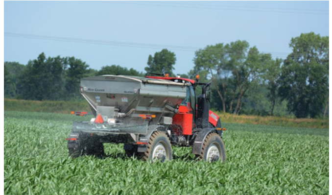
Figure 5. A red tractor pulling a granular fertilizer spreader applies nitrogen to an emerged corn field during a split application.
