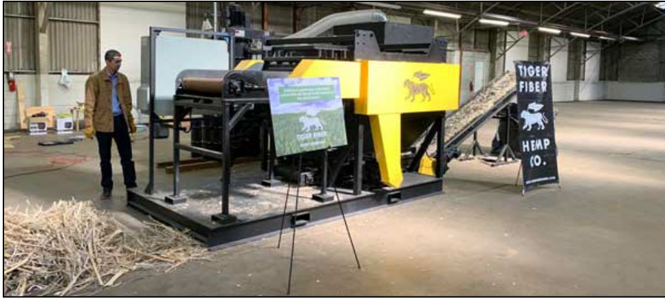
Exhibit 3.6.2 – Tiger Fiber Hemp Company Mobile Decortication Machine Prototype
