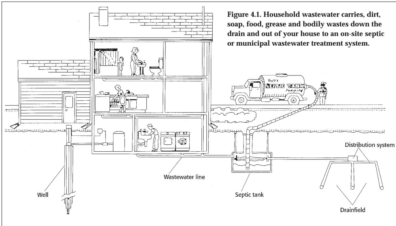
Figure 4.1. Household wastewater carries, dirt, soap, food, grease and bodily wastes down the drain and out of your house to an on-site septic or municipal wastewater treatment system.
