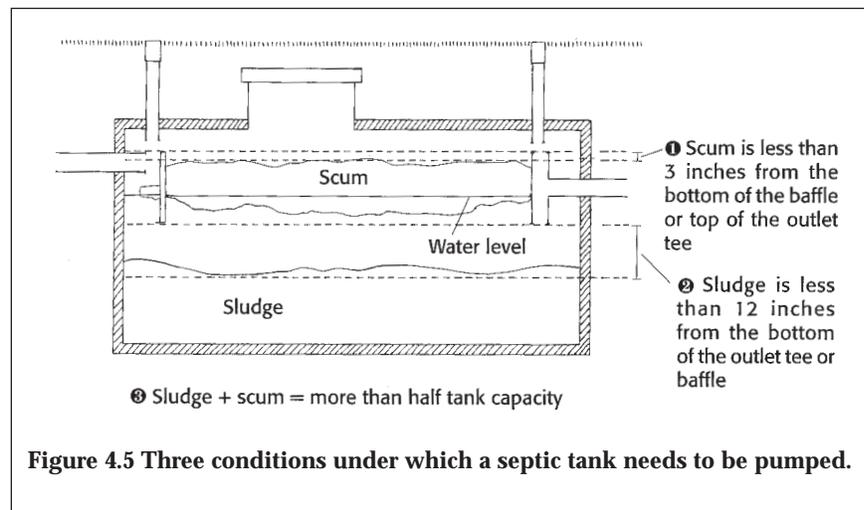
**Figure 4.5 Three conditions under which a septic tank needs to be pumped.**
