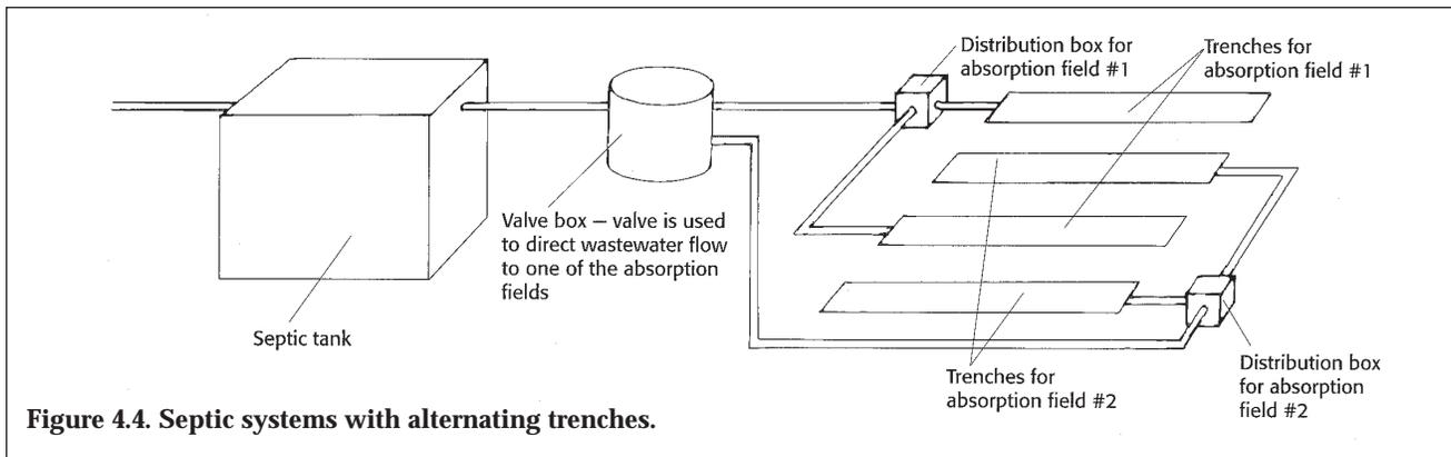
**Figure 4.4. Septic systems with alternating trenches.**
