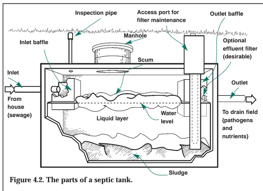
Figure 4.2. The parts of a septic tank.
