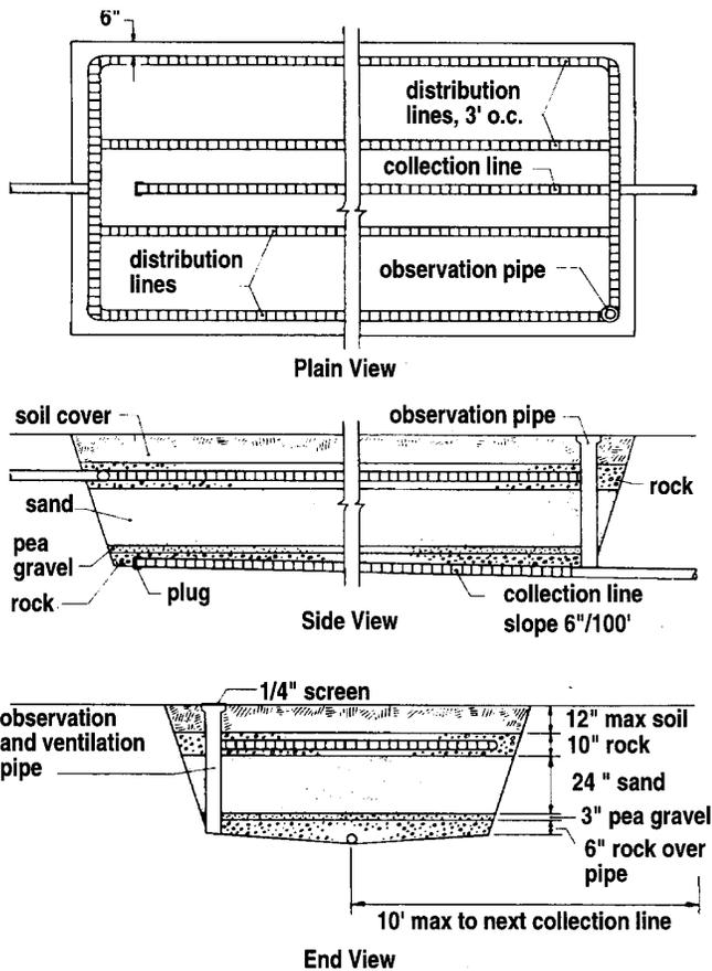
Figure 2. Buried sand filter. Source: *Onsite Domestic Sewage Handbook, MWPS24, Midwest Plan Service, 1982.*
