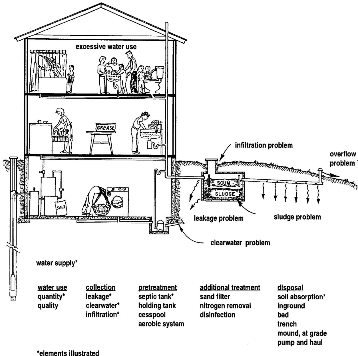
Figure 1. Typical household wastewater treatment system with problems. Illustration by Andy Hopfensperger, University of Wisconsin-Madison, Department of Agricultural Engineering.1 Overflow devices are not approved for installation in Missouri.
