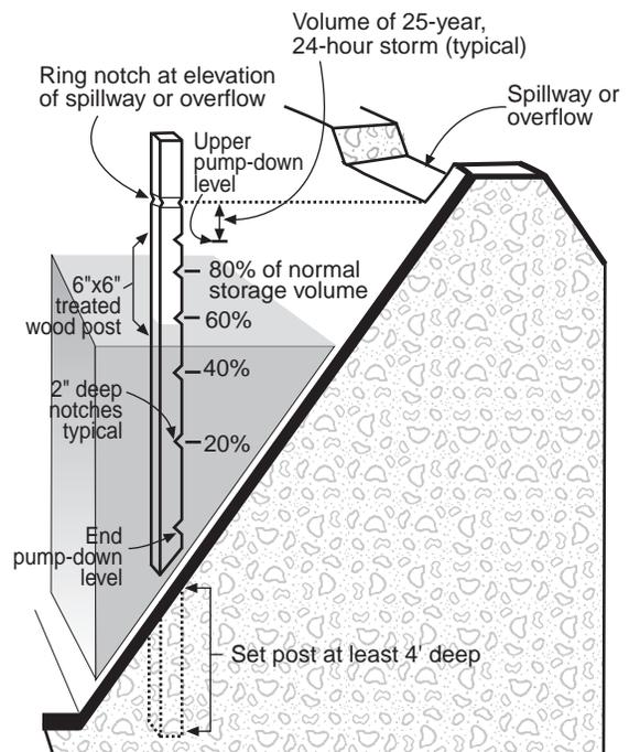
Figure 4. Pump-down marker in an anaerobic lagoon.
