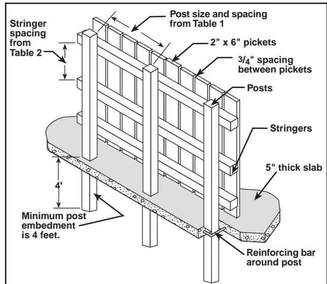
Figure 7. Typical construction details of a picket dam.
