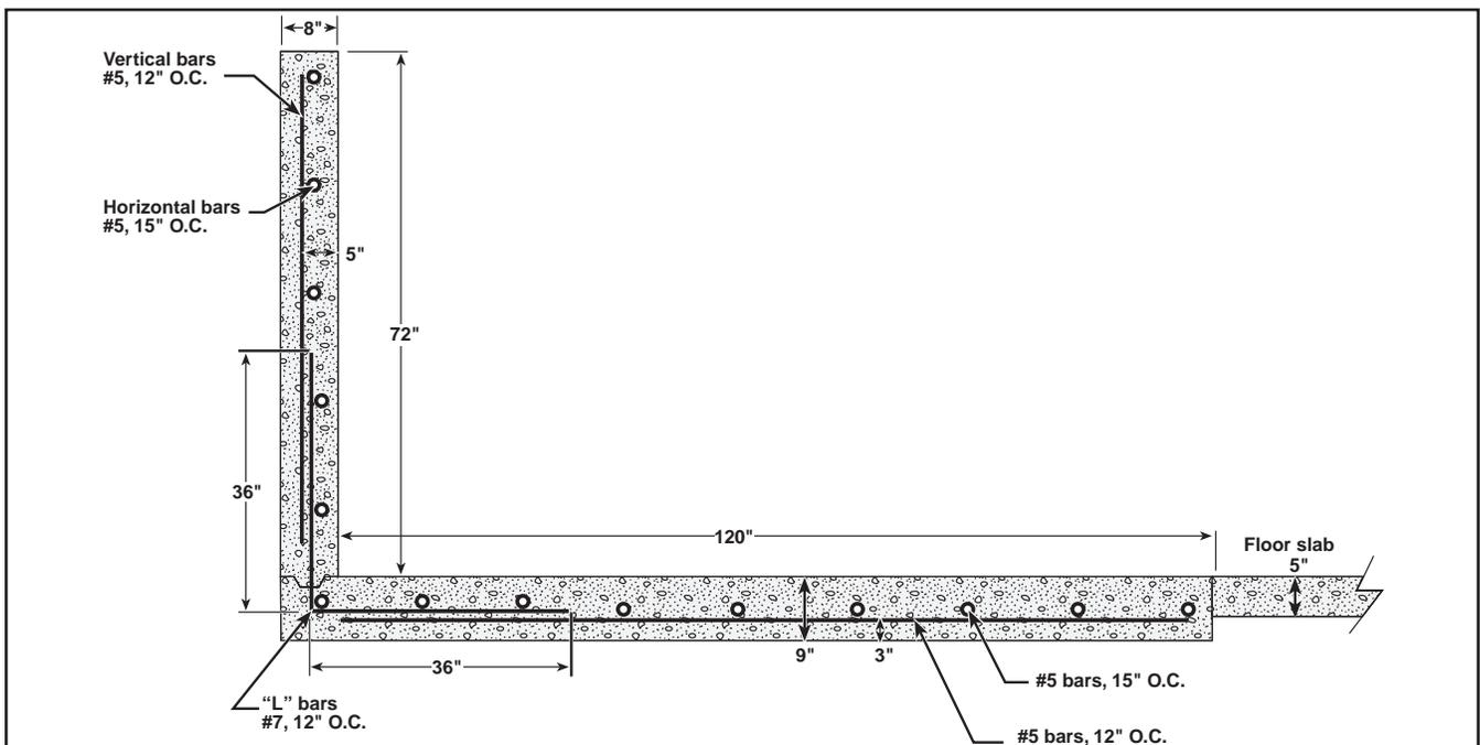
Figure 5. Design for a six-foot free-standing concrete wall.
