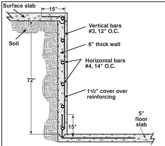
Figure 6. Design for a concrete wall tied into another slab.
