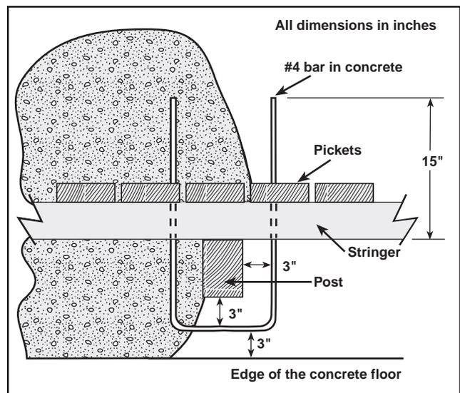
Figure 8. Reinforcement for posts in a concrete floor.
