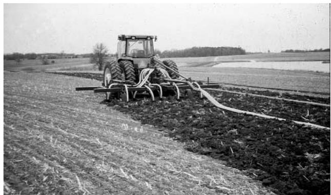
Figure 6. This drag-hose applicator can inject liquid and slurry below the soil surface.
