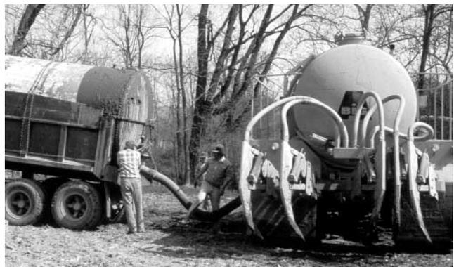
Figure 5B. The self-propelled, tank-type applicator shown in Figure 5A is being refilled from a tender truck.
