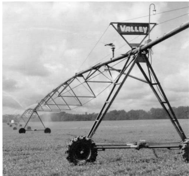
Figure 19. Center-pivot irrigator. Source: Valmont Slurry Manager.
