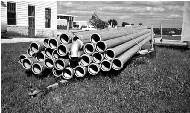
Figure 18. Portable aluminum pipe is available in a variety of sizes for use as a low-friction feeder conduit for irrigators and tractor-drawn, drag-hose applicators and injectors.
