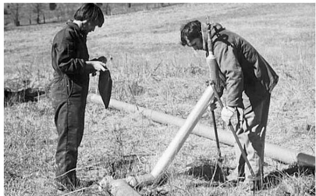
**Figure 15. Small hand-set sprinklers require more labor than other systems but may be more economical for small operations.**
