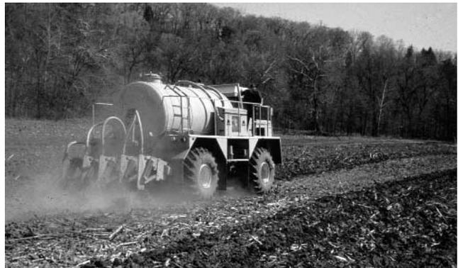
Figure 5A. This self-propelled, tank-type applicator is equipped to inject slurry below the soil surface, thus reducing nutrient losses and odor emissions.
