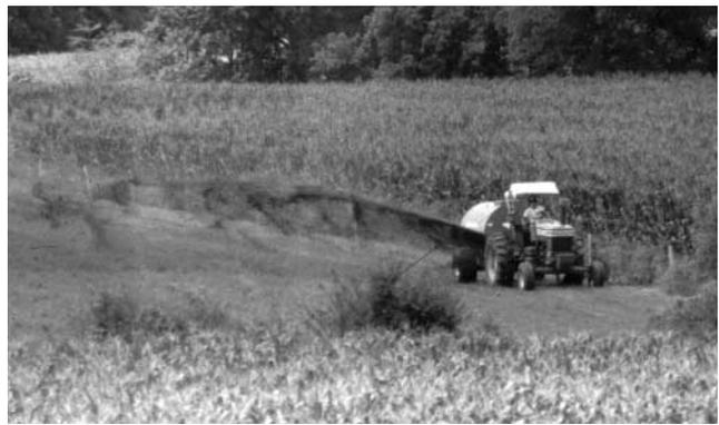
Figure 4. This tank-type applicator is broadcasting slurry onto the soil surface.
