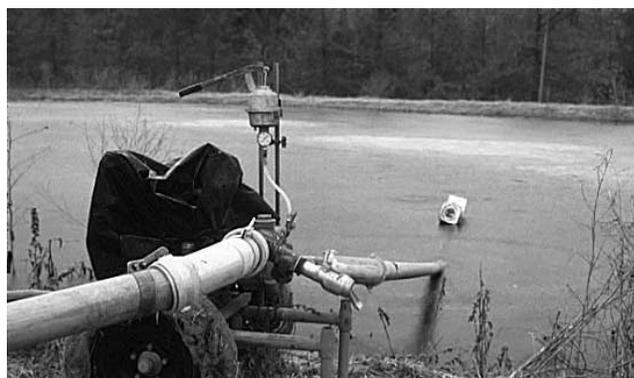
**Figure 9.** To prevent intake of floating debris, suspend an irrigation pump intake about 2 feet below the surface of a lagoon.
