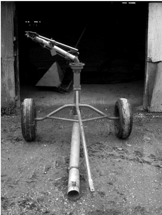
Figure 16. Stationary big gun on wheels to facilitate moving.
