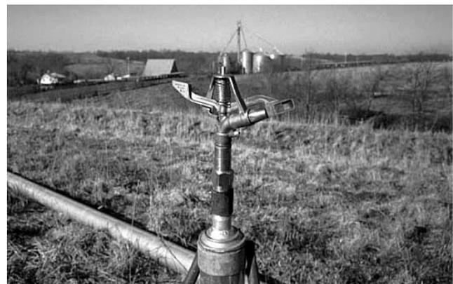
**Figure 14. Small sprinklers (up to ¾-inch diameter) can be used to irrigate lagoon effluent onto irregularly shaped fields.**
