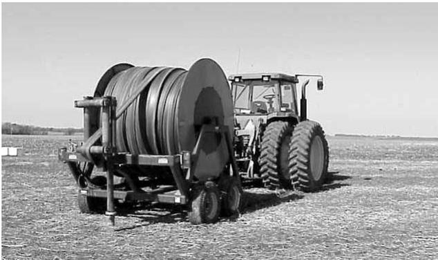
**Figure 12.** Hose carts provide a compact, fast means to transport, lay out and take up flexible drag hose or feeder hose.
