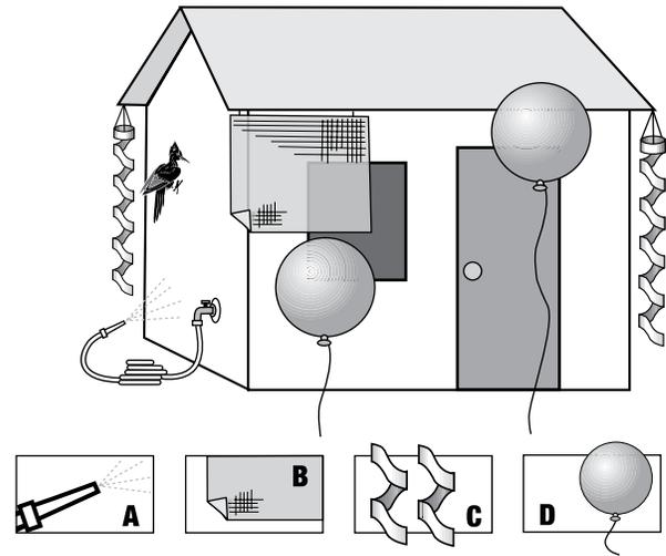
**Figure 2.** Woodpecker damage-control methods for structures: (a) high-pressure water hose, (b) fine-mesh netting, (c) highly reflective aluminum foil strips or Mylar tape, (d) helium-filled Mylar balloon.
