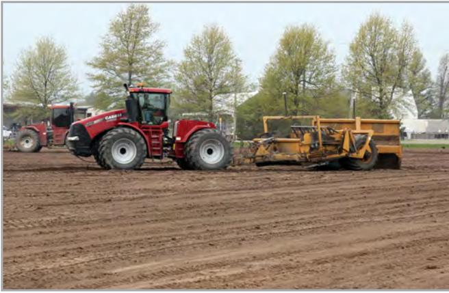
**Figure 22.** GPS guided land grading is used to improve drainage and uniformity of water application with furrow irrigation.
