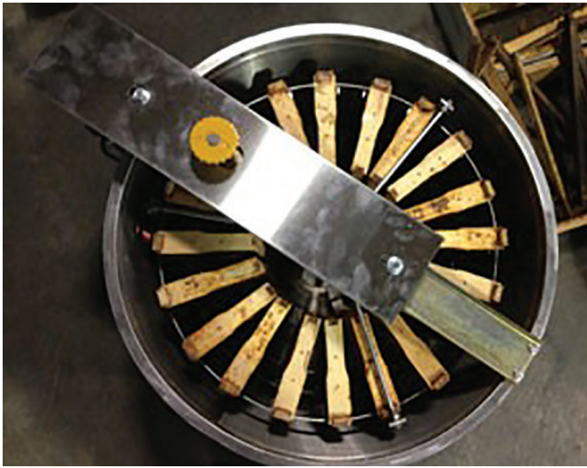
Figure 3. Radial extractor with frames placed in the reel like spokes of a wheel for removing honey from the comb (extractor shown here with cover removed). [E. H. Thorne (Beehives) Ltd.; used with permission]
