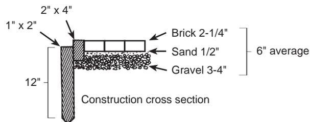
Figure 5. Cross section of patio or walk construction.
