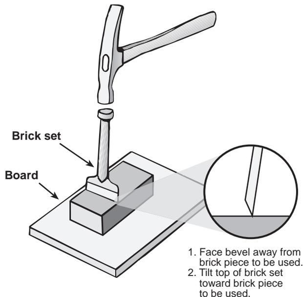
Figure 6. Using a brick set to cut brick.
