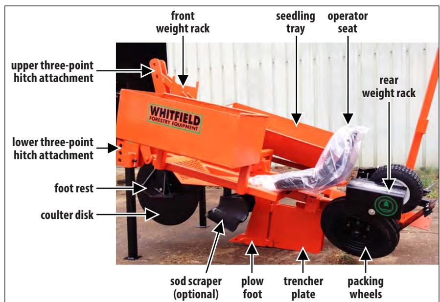
**Figure 11.** A typical mechanical tree planter.
