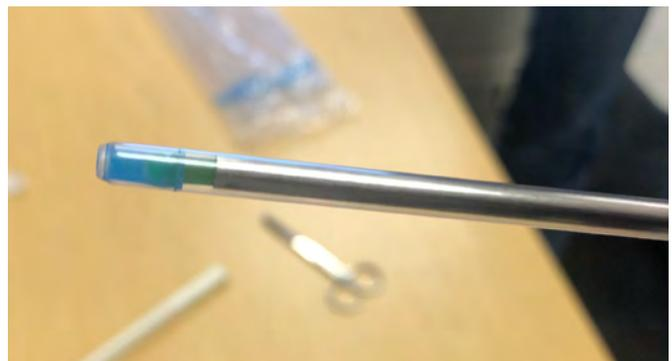
**Figure 7.** A plastic sheath with its tip appropriately locked in place over the straw and catheter.
