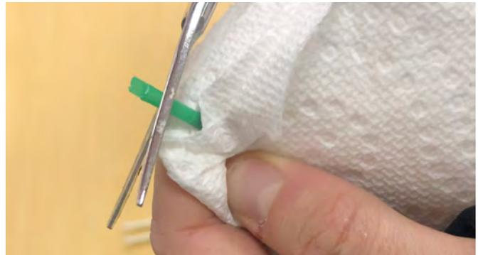
**Figure 6.** Cutting the sealed end of the straw at a 90-degree angle.
