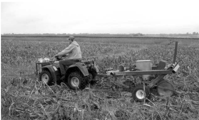
Figure 2. An all-terrain vehicle with a one-row, no-till planter makes an economical way to seed a vegetative barrier.
