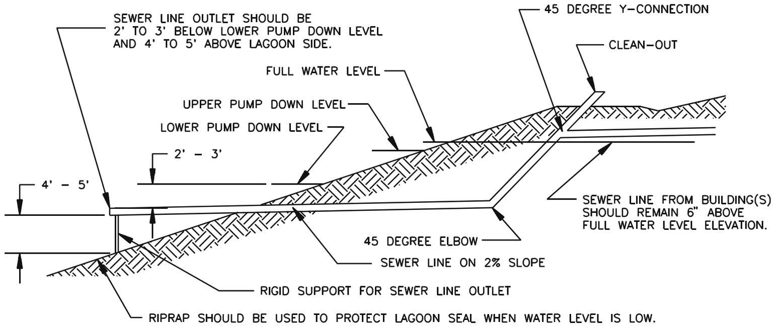
Figure 6. Scaled Sketch of Submerged Inlet into Anaerobic Lagoon.
