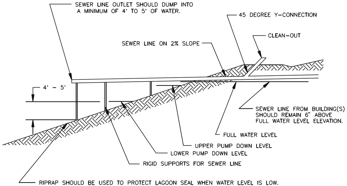
Figure 7. Scaled Sketch of Surface Inlet into Anaerobic Lagoon.
