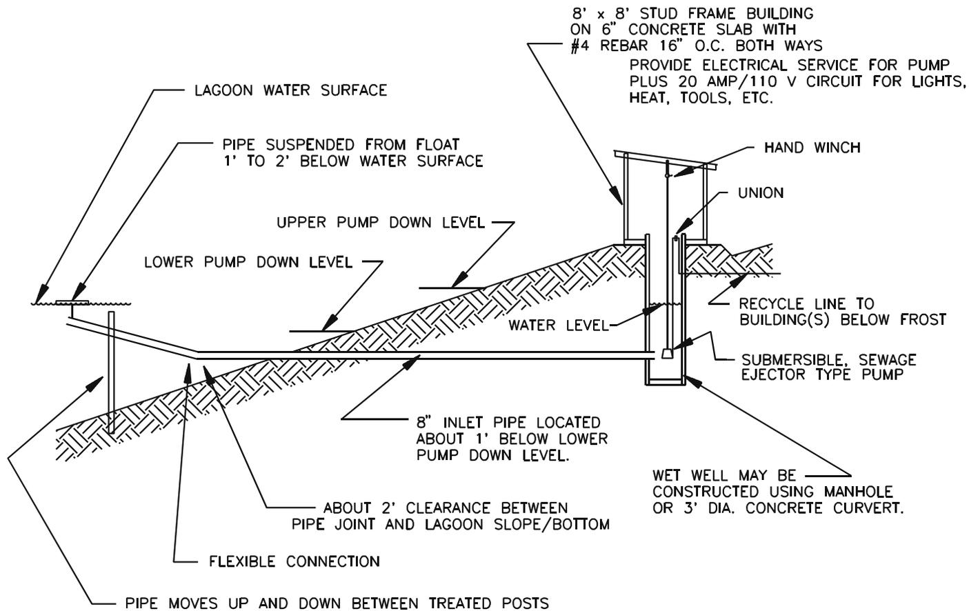
Figure 8. Scaled Sketch of Wet Well Installation for Lagoon Recycle Pump.
