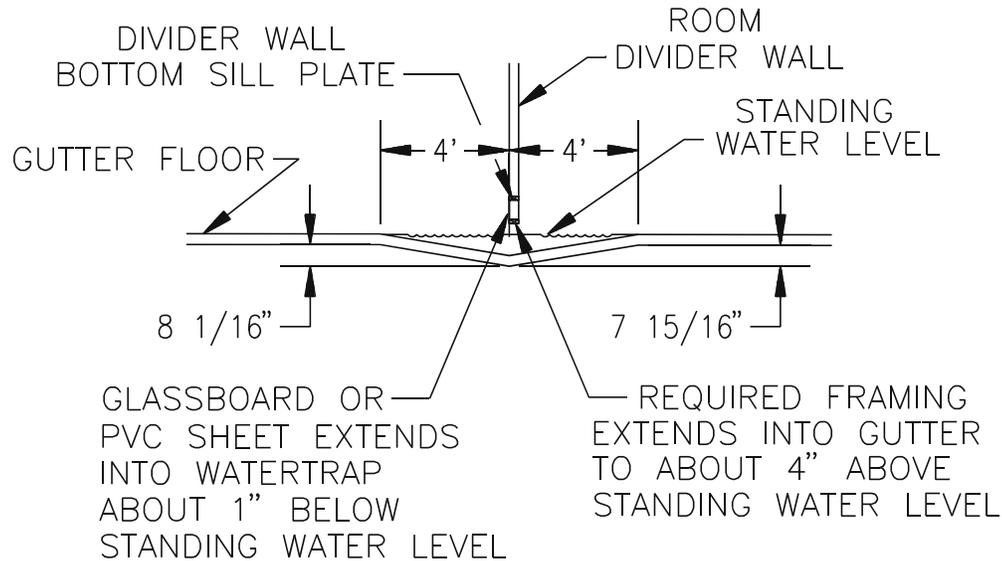
Figure 6. Scaled Sketch of Flush Gutter Water Trap
