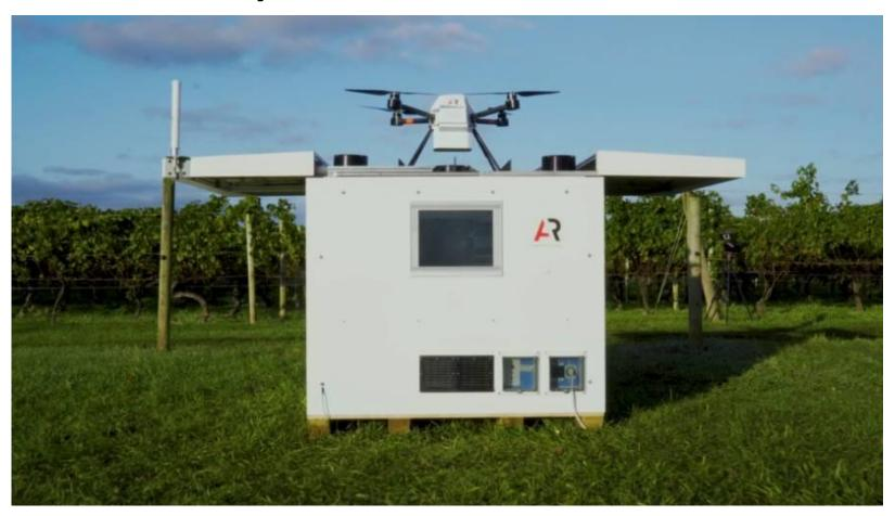
American Robotics, an industrial drone developer specializing in agricultural automation, has unveiled its flagship product Scout. It is a self-charging, self-managing drone system capable of autonomously carrying out daily scouting missions.
