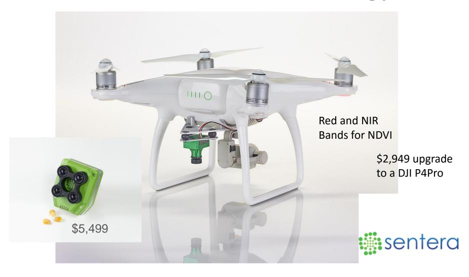
DJI Phantom 4 with Sentera Single NIR Sensor and Standard RGB Camera
