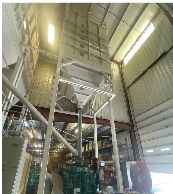
Scales, which can be used in place of the flow meters for lower volume applications.
