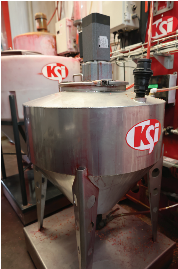
Chemical Hopper. This is another scale station with a permanent chemical hopper. This station is used for smaller components with a lower use-rate.
