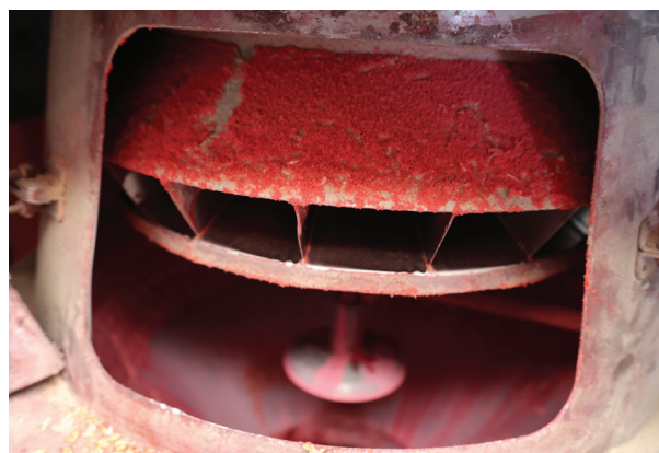
Closeup of the seed diffuser, with the atomizer disk below (small disk hanging underneath).
