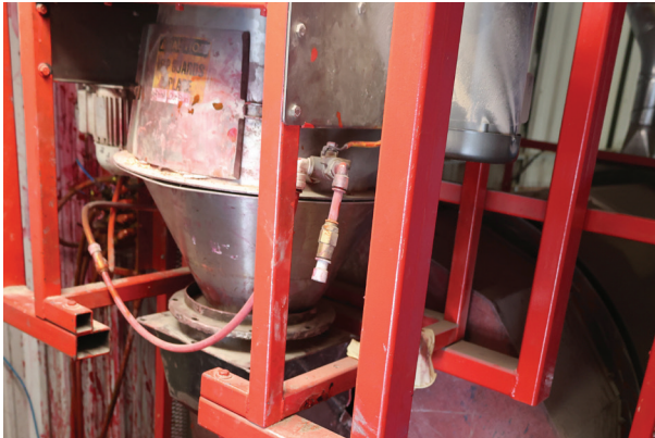
Atomizer. Chemical is pumped into the atomizer and onto a spinning wheel. The spinning wheel creates a mist of chemical. A steady flow of seed falls on all sides of the spinning atomizer disk which enables each seed to get initial contact with the chemical treatment. (All of this occurs within the atomizer).
