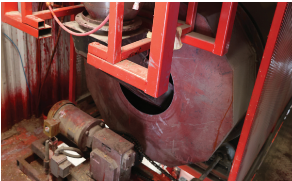
Treater Drum: From the atomizer, the wet seed is tumbled through the drum. Tumbling serves to distribute an even coat of chemical to the surface of the seed.
