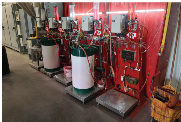
Weigh scales on a direct-injection seed treating system. Each scale weighs a different treatment component. The system injects individual chemical components using a loss-in-weight method.
