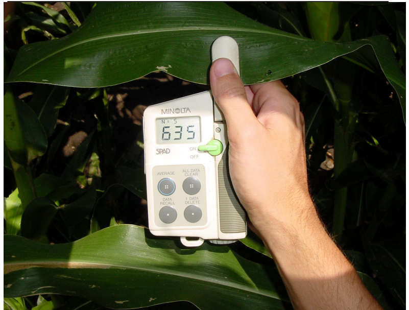
Figure 10. Hand-held chlorophyll meters are clamped over a leaf to measure light transmittance through a leaf.
