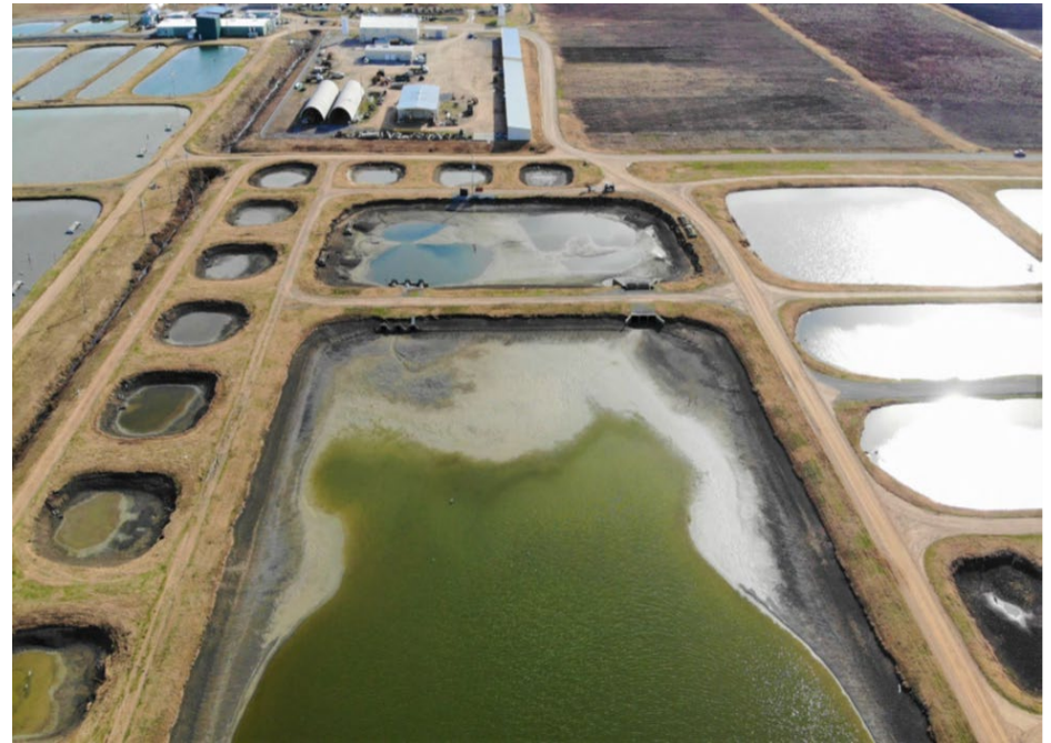
Seven-Acre Split-Pond without Levee in Five-Acre Waste Treatment Zone using Paddlewheel Delivering 10,000 to 15,000 gpm Water Flow (9.4-6.3 hrs cycle time, \sim 0.0 - 0.06 fps)
