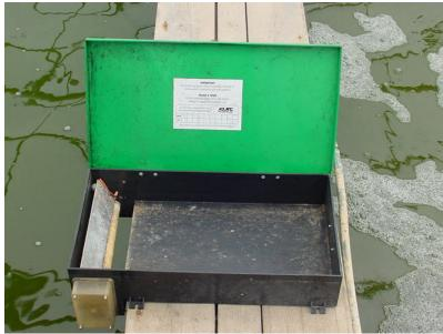
Belt feeders for continuous feed addition improves water quality
