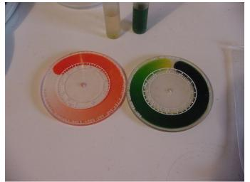
"Hach" fish-farmers kit, colorimetric wet chemistry Requires clean lab area, distilled water
