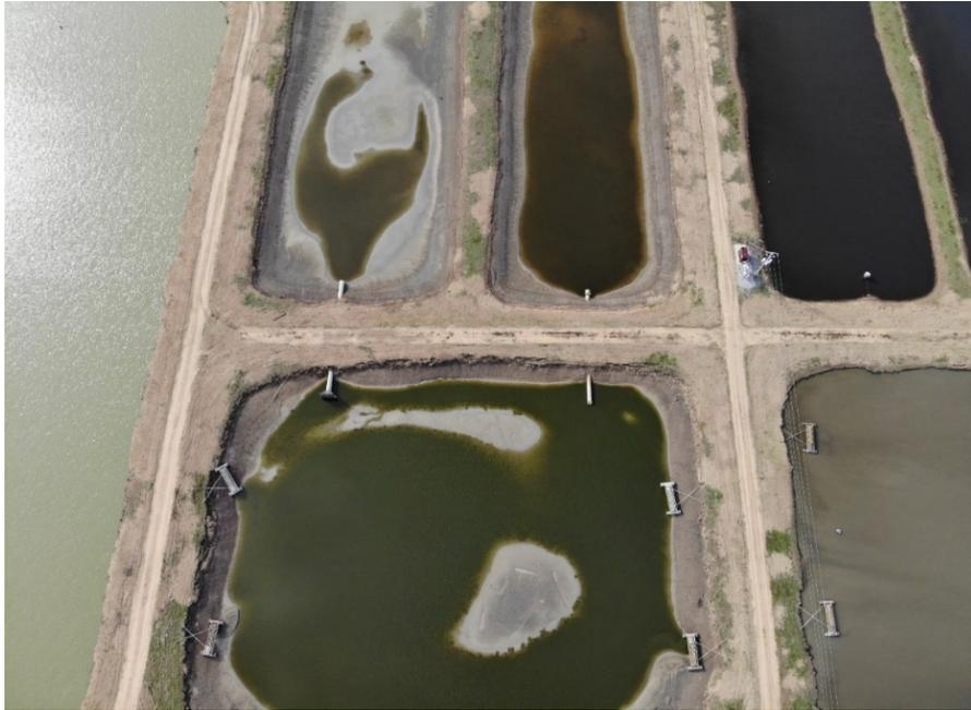
Seven-Acre Split-Pond **with Levee** in Five-Acre Waste Treatment Zone using **Culvert Pumps** Delivering **8,000 gpm** (11.8 hrs cycle time)
