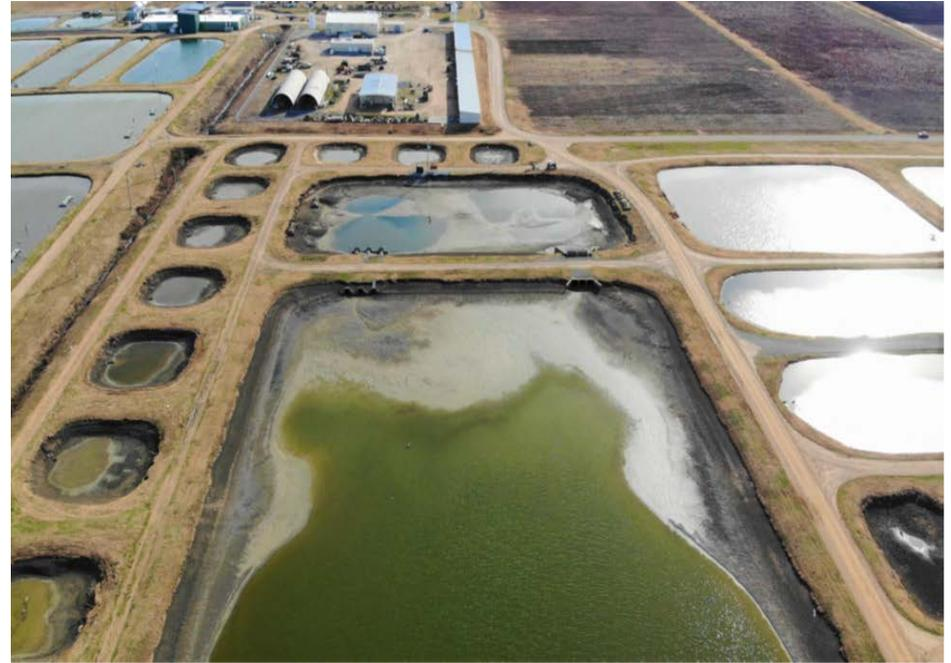
Seven-Acre Split-Pond **without Levee** in Five-Acre Waste Treatment Zone using **Paddlewheel** Delivering **10,000 to 15,000 gpm** Water Flow (9.4-6.3 hrs cycle time)
