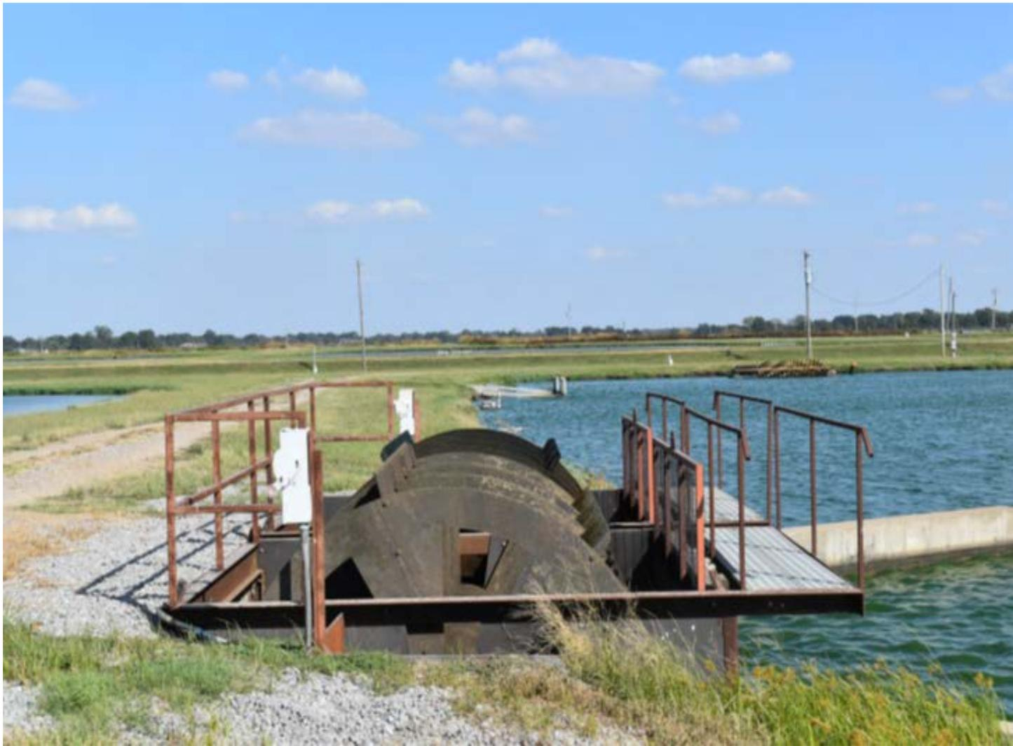
**Paddlewheel Used to Move Water in Split-Pond Without Central Levee.**
