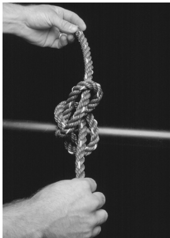
6. For added assurance, put the free end of the rope through the last loop.
