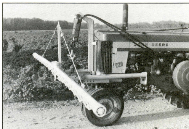
Figure 5. Use a high carbon steel tube (drill stem) frame to eliminate twisting. The cable and pulley double the 8-inch cylinder stroke for 16 inches of boom height movement.
