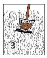
Tilt the shovel back and lift out the soil slice
