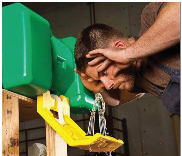
Figure 5. Water for eye flushing must be available for handlers when using a pesticide that requires eye protection. Haws Corporation photo.
