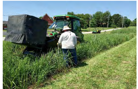
Figure 1. PaddockTrac sensor calibration harvest on native warm season grass plots at UCM-Warrensburg.
