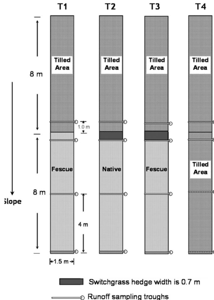
Fig. 1. Schematic diagram showing vegetative buffers and control.
