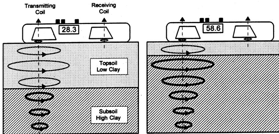
Fig. 1. Schematic showing operation of the Geonics EM38 soil conductivity sensor in vertical dipole mode over deep topsoil (left) and shallow topsoil (right).
