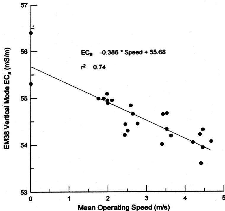
Fig. 9. Sensitivity of  $EC_a$  measurement to changes in operating speed.
