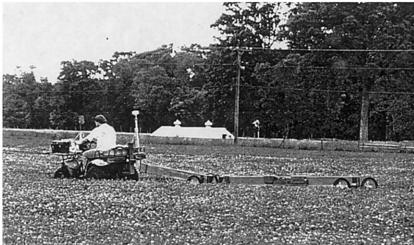
Fig. 3. Mobile  $EC_a$  measurement system incorporating Geonics EM38, GPS receiver, data logging computer, and ATV.
