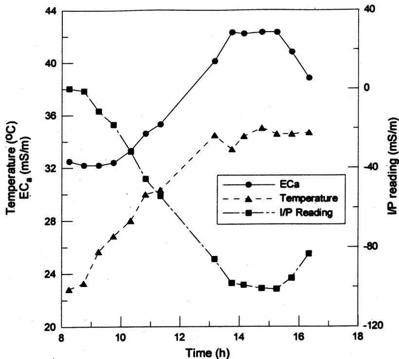
Fig. 5. Change in  $EC_a$ , I/P reading, and ambient temperature over time in fixed point drift experiment.
