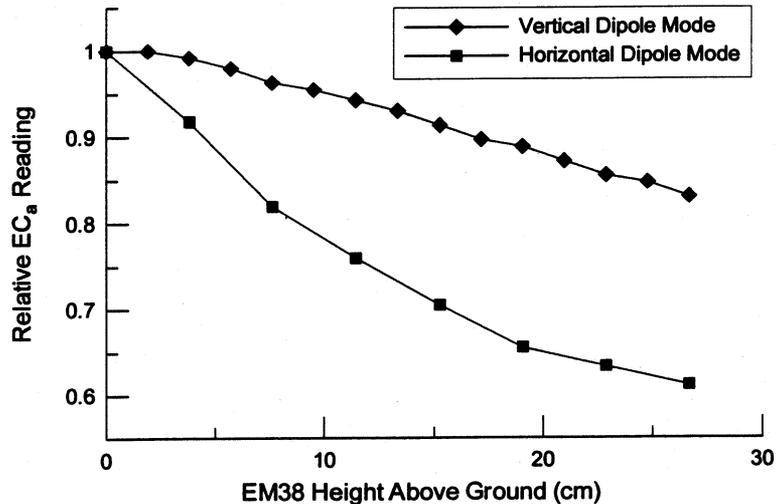
Fig. 10. Effects of changes in sensor height on EC<sub>a</sub>.
