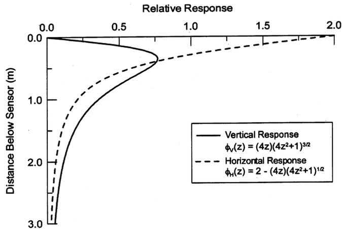
Fig. 2. Relative response of EM38 sensor as a function of distance (adapted from McNeill, 1992).
