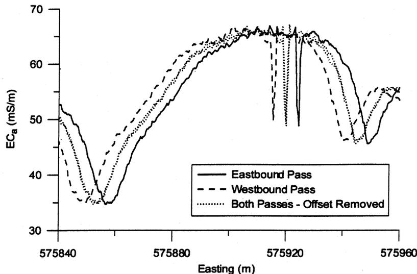
Fig. 7. Paired data collection runs at 1.9 m/s, showing position offset in the  $EC_a$  response caused by traversing a metal pipe, and correspondence of the two runs after removing the offset.
