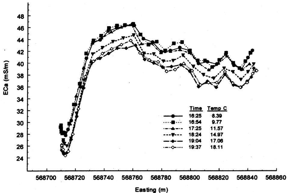
Fig. 4. Repeated  $EC_a$  measurements over a calibration transect, showing instrument drift over time.
