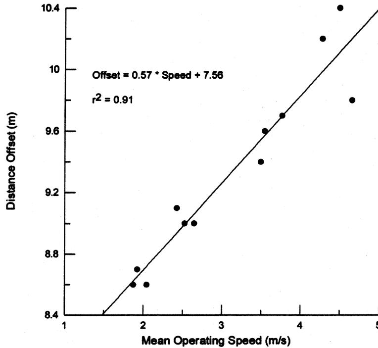
Fig. 8. Position offset between paired  $EC_a$  data collection runs as a function of operating speed.
