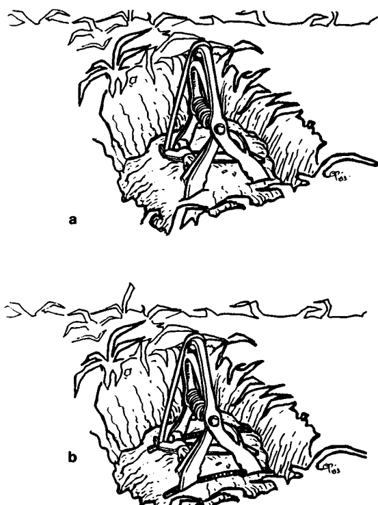
Figure 9. (a) The scissor-jawed trap is set so that the jaws straddle the runway. (b) In heavy soils, make a path for the jaws to travel so they can close quickly.
