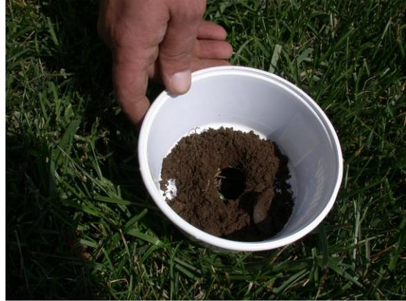
**3. The plastic tub catches the soil as the bit is extracted from the hole**
