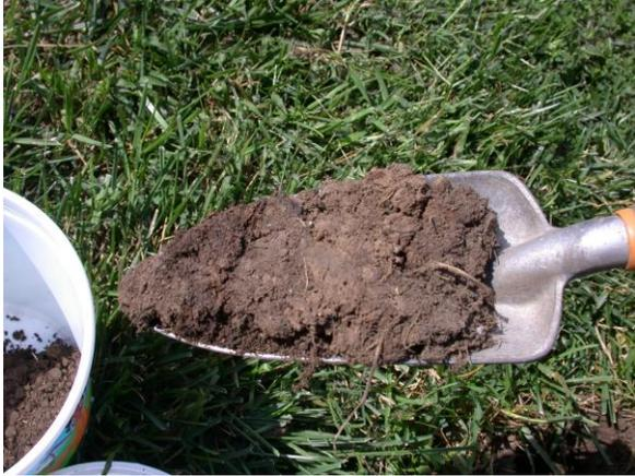
**8. A slice of soil about 1" thick from the side of the hole**
