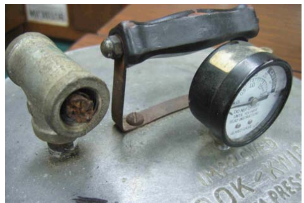
This homeowner was using a stick and pipe tee to try to regulate pressure on her food canner, potentially putting her family at risk for botulism poisoning from underprocessed canned goods.
