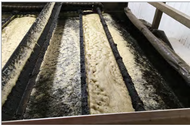
Figure 28. DAF froth discharge to MD presses.
