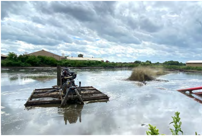
Figure 2. PTO-drive lagoon agitators and agitation boat in action.
