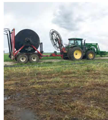
Figure 6. Booster pump (left), application toolbar and tractor (center), and hose cart and humper (right).
