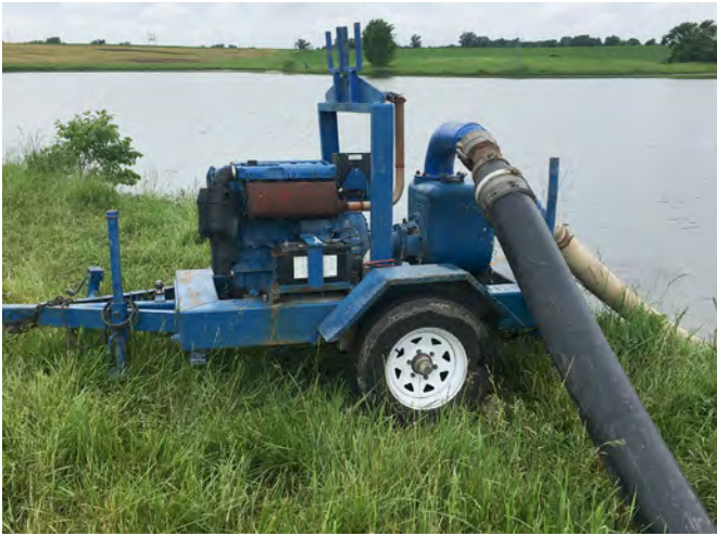
Figure 5. A dilution pump was used to pump water from the nearby lake (left) to the dairy lagoon (right) with agitation boat and lagoon agitation working in the background.
