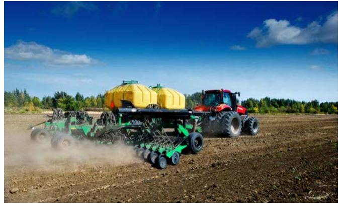
Figure 4. Air seeders offer a solution to the trade-off between seeding accuracy, work rate, and a combined fertilizer application.
