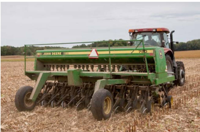
Figure 3. A no-till box-type drill is a good solution for uniform emergence at a low cost. Photo courtesy of Edwin Remsberg and USDA–SARE.
