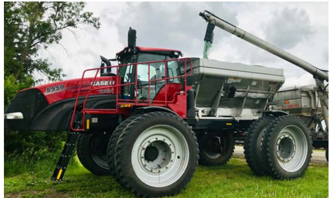
Figure 9. High clearance spreaders can straddle crop rows to spread seed and fertilizer over growing crops.
