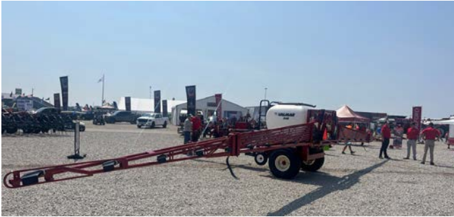
Figure 5. An air boom spreader can be a quick and effective way to seed a variety cover crops.
